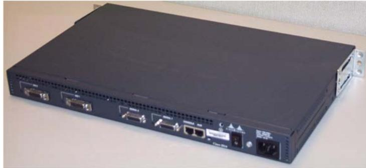
Figure 3. Cisco 2514 router with two Ethernet ports and two serial ports.
