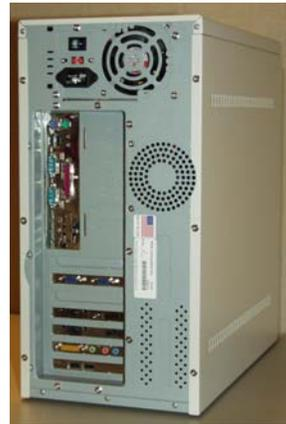
Figure 2. Ports in the back of a PC.
