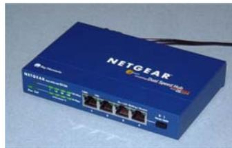
Figure 4. Ethernet Hub with four ports.
